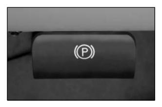
To release the parking brake, hold the regular brake pedal down. Pull the bottom edge of the lever, located above the parking brake pedal to release the parking brake.
